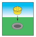
If you desire to remove the DARTZ<sup>™</sup> ground sleeves, place the tip of a shovel or other tool underneath the top lip of the sleeve and use leverage to pry it up. There is a slot in each fin to continue prying up. You may need to dig around the sleeve to help loosen it.
